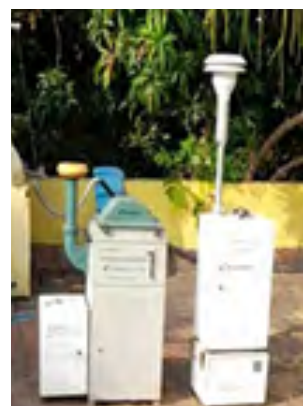
AAQ Station installed in Umangalam, Neyveli
