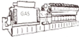
Gas - Up to 25 MVA
