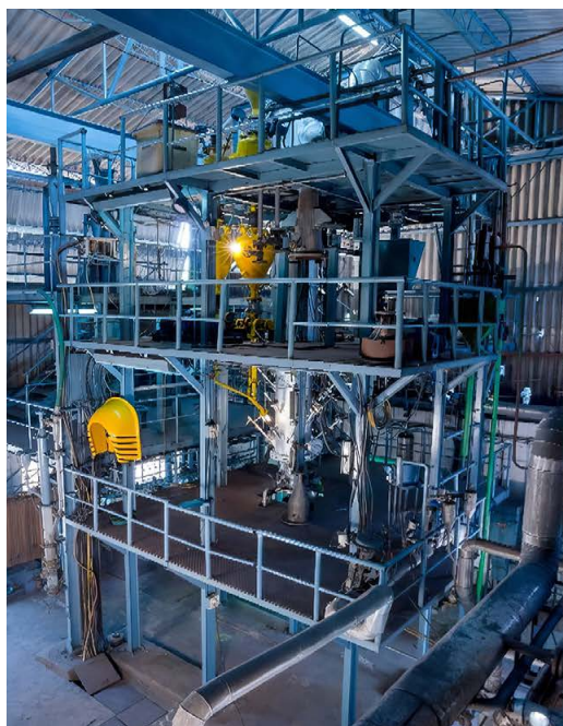
1.2 TPD Coal Gasification pilot plant for producing 0.25 TPD Methanol from high-ash coal established by BHEL at Hyderabad
