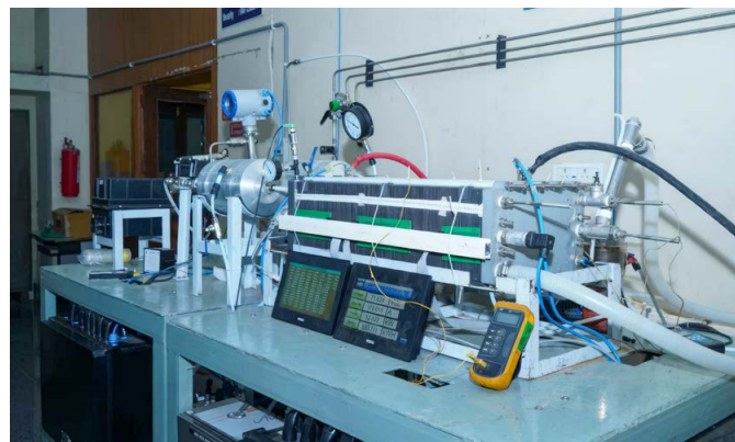
Fuel cell stack performance evaluation, under diverse test conditions, at Corp. R&D, Hyderabad
