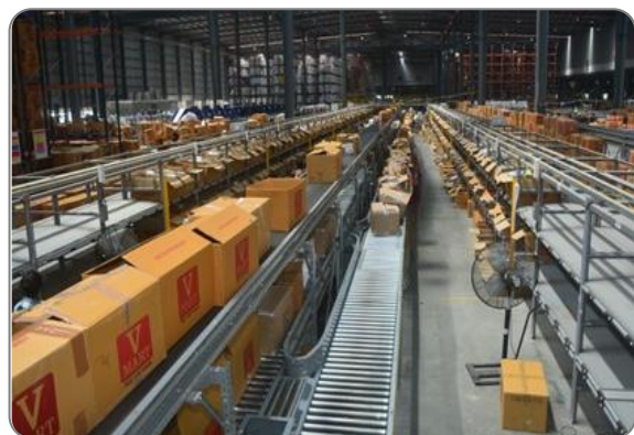
Automated workflow using scanners and conveyers
