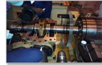
228MW, STEAMTURBINE,SABIYA, KUWAIT, MAIN OIL PUMP OVERHAULING
