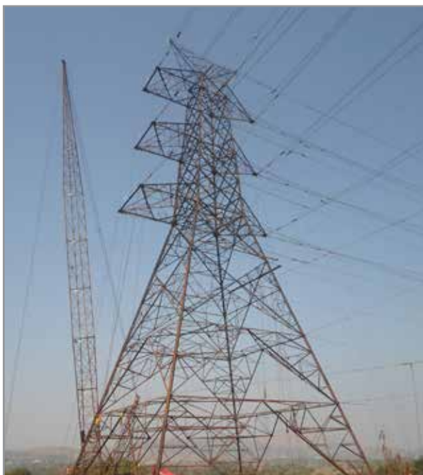
SAM 8414:- 400kV D/C 4D90 (60°-90°)/4DT(0°-45°) tower tested for end client- GCCIA and Consultant - Energoprojekt ENTEL
