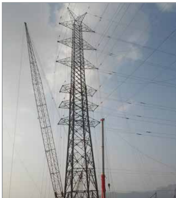
SAM 8283:- 400-220kV M/C 'MD' (30°-60° Dev) tower tested for end client - JSW Steel Limited and Contractor - BNC Power Projects Limited
