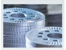
Produces laminations from 50 mm to 1,250 mm outer diameter
