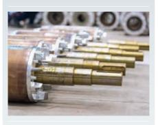
Supplies ready-to-use assembled rotor cores with stacking under hydraulic pressure
