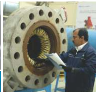
Boiler Circulation Pump rewinding
