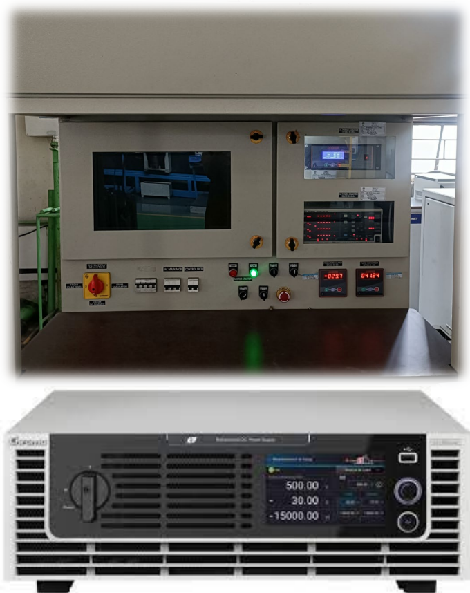
Solar Pump Performance Test Panel with Solar Simulator
