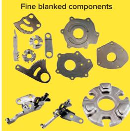
Fine blanking produces close tolerance parts from materials of higher thickness. Cut edges are 100% free of tear and in most cases parts are suitable for mechanical function without the need for subsequent machining. This technology enables production of "Near net Shape" and even ready to assemble sheet metal parts.
