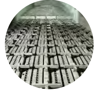
First in India to install Cross bar cooler to reduce specific fuel consumption
