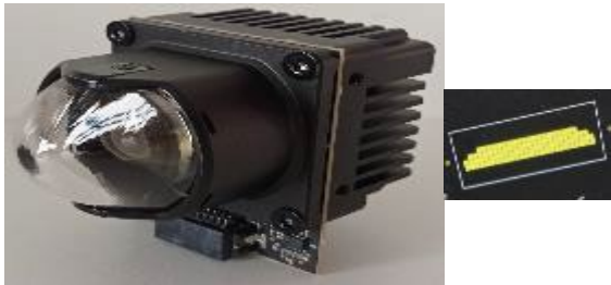
Matrix (ADB) Headlamp Module and Controls
