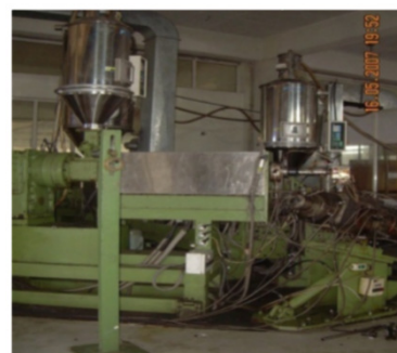
CCV Line (Involving Dry Cure Dry Cool technology) For manufacturing HT Cables Up to 132 kV
