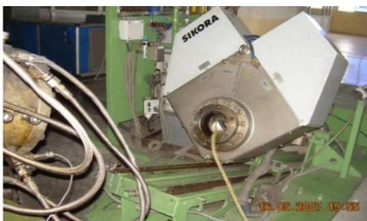
Sikora Online X-Ray Machine Used for Monitoring Product Quality
