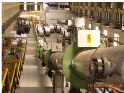
CCV Line (Involving Dry Cure Dry Cool technology) For manufacturing HT Cables Up to 132 kV
