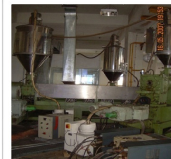
CCV Line (Involving Dry Cure Dry Cool technology) For manufacturing HT Cables Up to 132 kV
