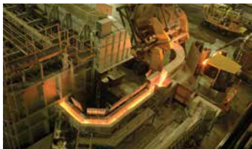
Molten Aluminium being poured in Casting machine in Jharsuguda Plant
