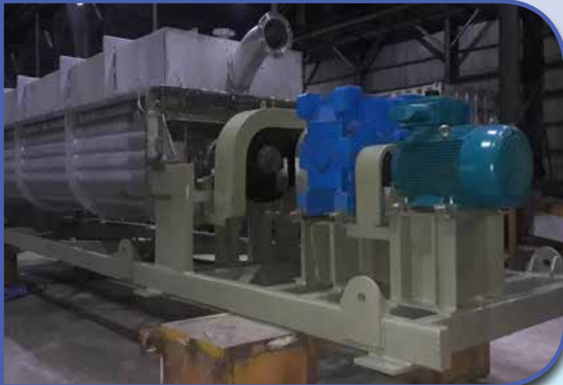
PADDLE DRYER - DIRECT COUPLED DRIVE
