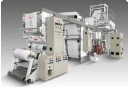
FOILEX™ - Monolayer Blown Film Lines
