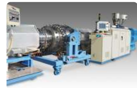
FLOWEX® - Twin Screw PVC Pipe Plant
