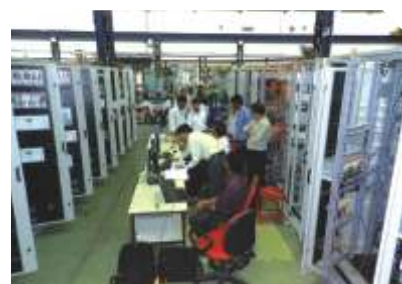
Customer inspection during integrated FAT (Factory Acceptance Test) at Pallavaram unit for Control relay panels
