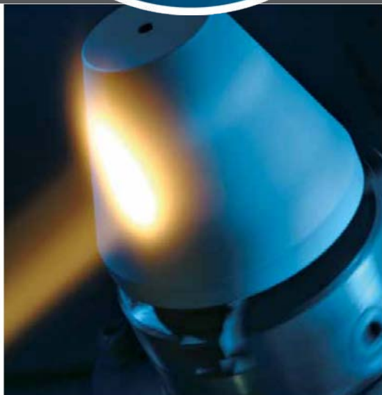
Thermal spraying for optimal metal coating.
