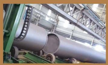
Jindal SAW Limited is the market leader in India for manufacturing large diameter Submerged Arc Welded (SAW) pipes. This particular type of pipe is primarily used in transportation of oil, gas, slurry and water.
