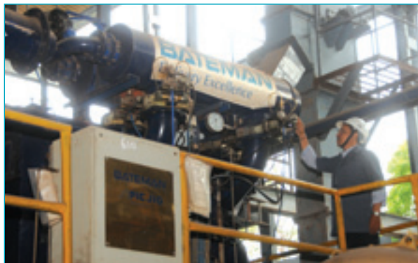
Jig - a gravity preconcentration/ concentration unit at R&D Centre
