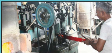
Making Press Beads from Semi Automatic machines
