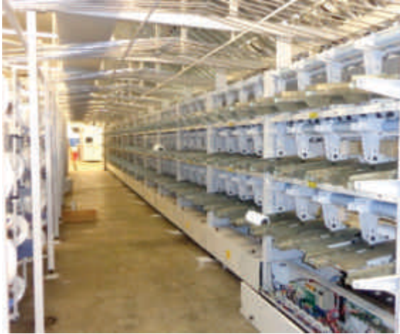
ANOTHER AUTODOFF MACHINE BEING ERECTED
