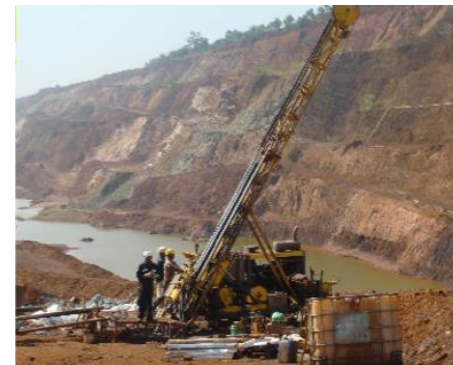
Core drilling for Chromite for Tata Steel Limited
