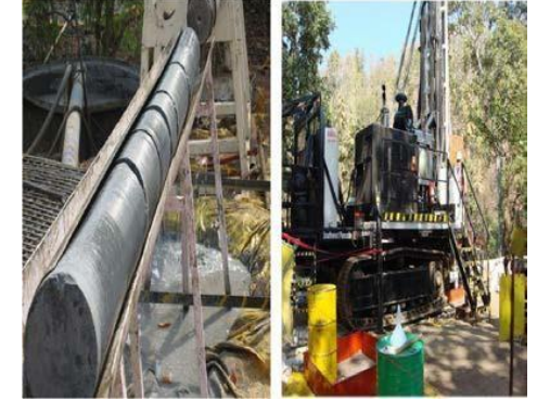
Large Diameter Kimberlite core (8") for Rio Tinto at Bunder, MP – Drilled by BLY LF230 upto a depth of 352 Meters. Largest coring done in India till date
