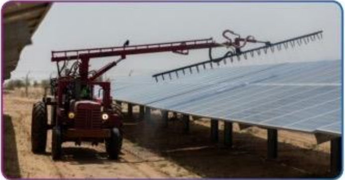
Innovation in Module Cleaning System (Semi - Automatic)
