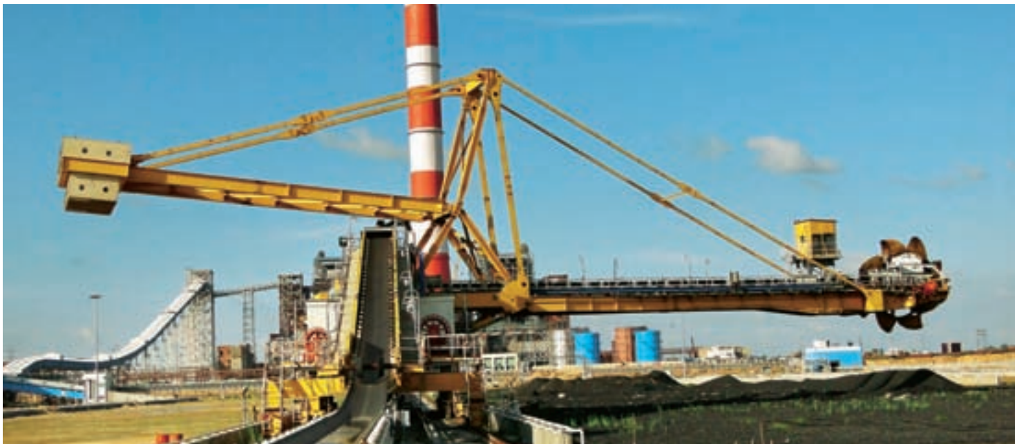
Open stockyard equipped with rail-mounted stacker reclaimers at India's multi-purpose river valley project for Damodar Valley Corporation's Koderama Thermal Power Project in Jharkhand.
