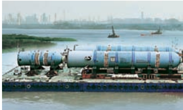
Cr-Mo-V forged reactors being despatched by barge from L&T's captive jetty at Hazira for Kuwait National Petrochemical Corporation's Clean Fuels Project.
