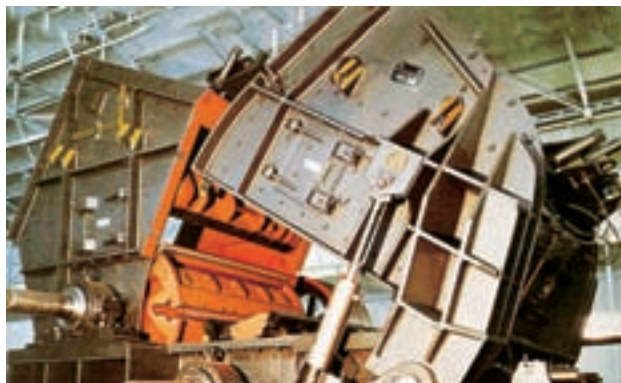
Limestone crusher manufactured at L&T's Kansbahal Works.
