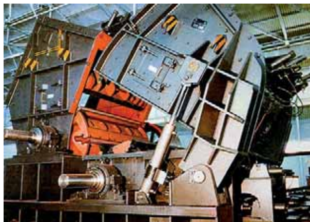
Limestone crusher manufactured by L&T.
