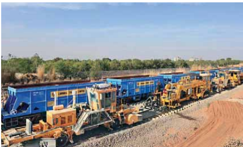
The new track construction machine is capable of laying 2 km of tracks per day, setting a benchmark in high-speed rail construction on the Western Dedicated Freight Corridor project.
