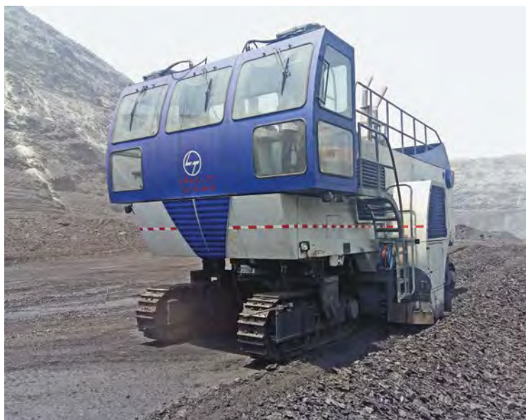
L&T's KSM-404, the largest surface miner in Indian coal mine at Gevra, Chhattisgarh
