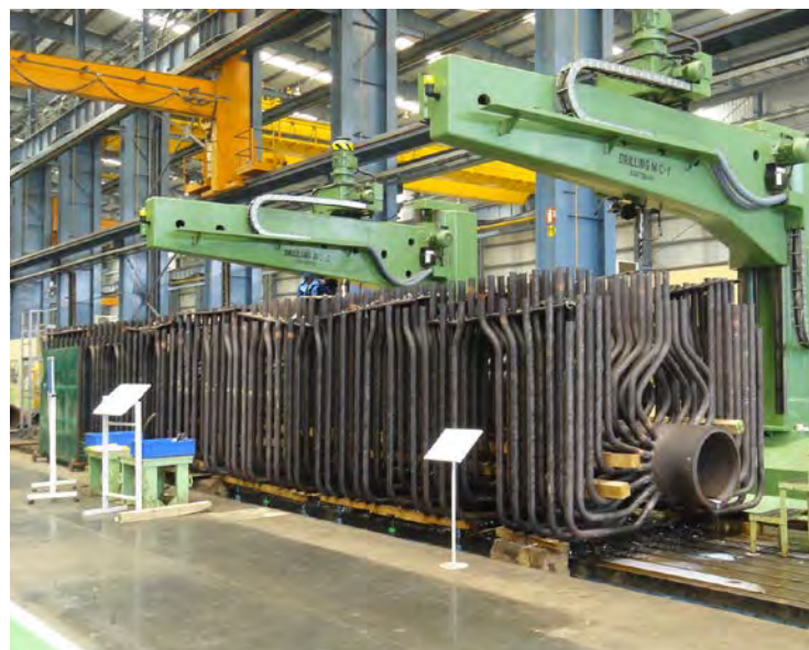
Boiler internals being manufactured at Hazira, Gujarat
