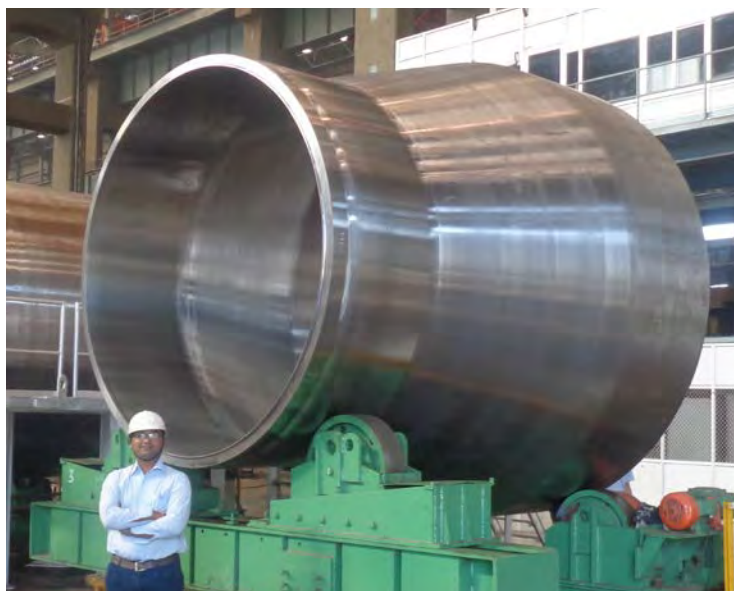
Nuclear Steam Generator Cone Shell - 16 MT
