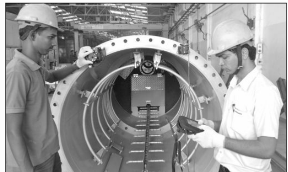
Employees using world class laser equipment for the inspection of wind mill tower flange flatness
