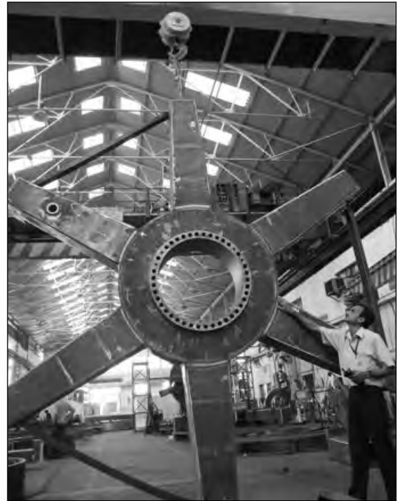
Manufacturing of Stator carrier of wind turbine parts having capacity of 800 KW - 1.2 MW
