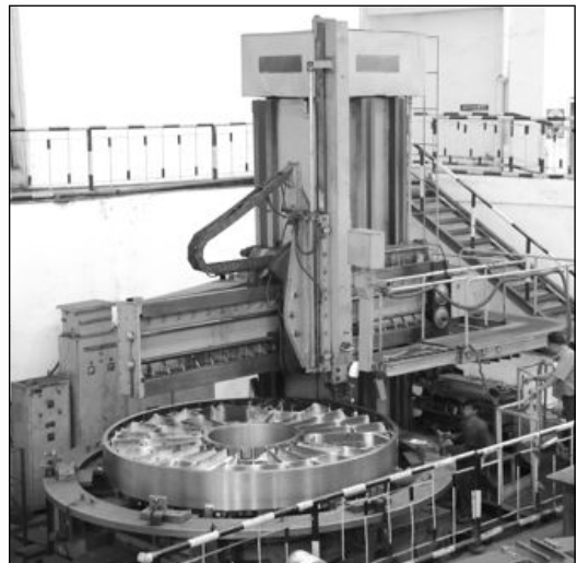
Precision machining of wind turbine parts on Premier's own made CVBM (Vertical Turning Lathe)
