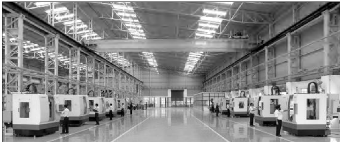
CNC Vertical Machining Centres under testing
