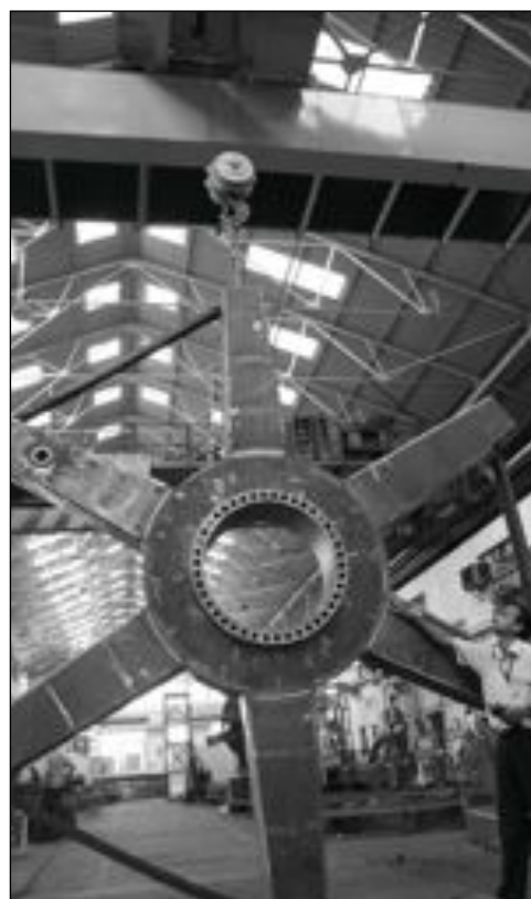
Manufacturing of Stator carrier of wind turbine parts having capacity of 800 KW - 1.2 MW
