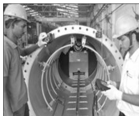
Employees using world class laser equipment for the inspection of wind mill tower flange flatness
