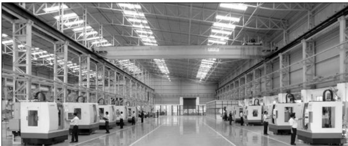
CNC Vertical Machining Centres under testing
