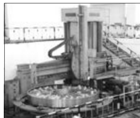
Precision machining of wind turbine parts on Premier's Vertical Turning Lathe
