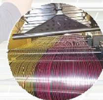
E-beam irradiated cables
