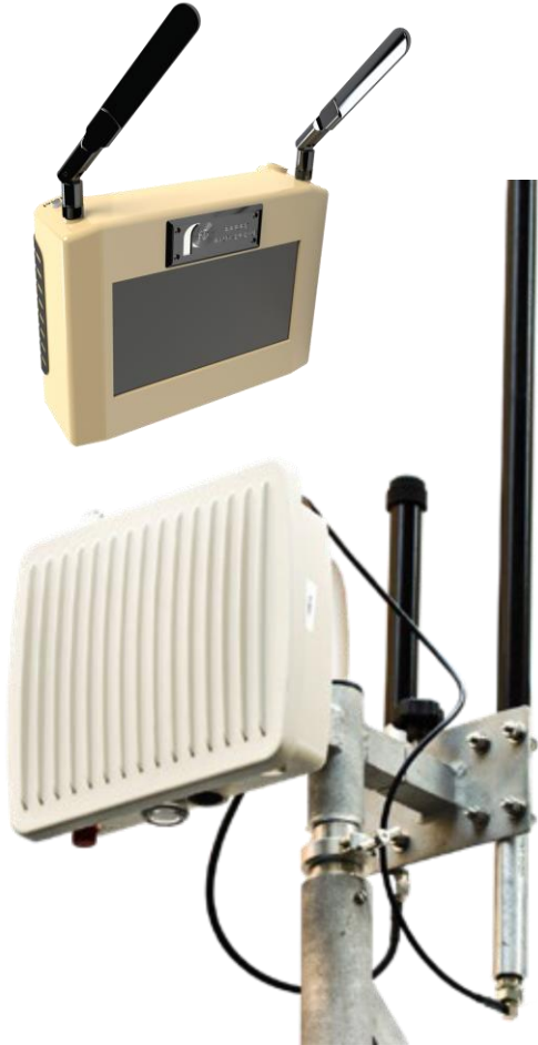
Hydra & Sky Sense Drone Detection Systems
