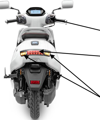
LED Tail Lamp with Stop Lamp
