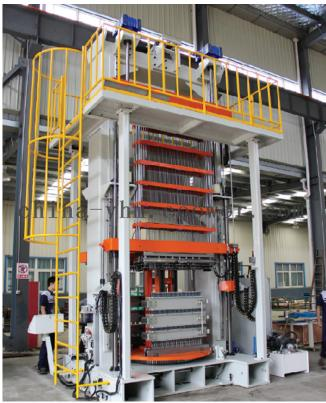
The 5 mm Fin Press and Vertical expander machines were installed the Himachal Pradesh Plant to produce the recommended 5 mm coils, which are used in some models instead of the older 7 mm coils
