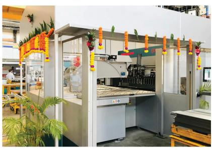
The new Salvagnini Px installation at Dadra Plant efficiently bends sheet metal for product chassis, thereby increasing the capacity of the Plant
