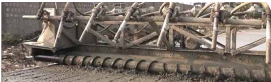
Sensor Paver technology – laying concrete roads up to 7 meters wide using sensor paver technology
