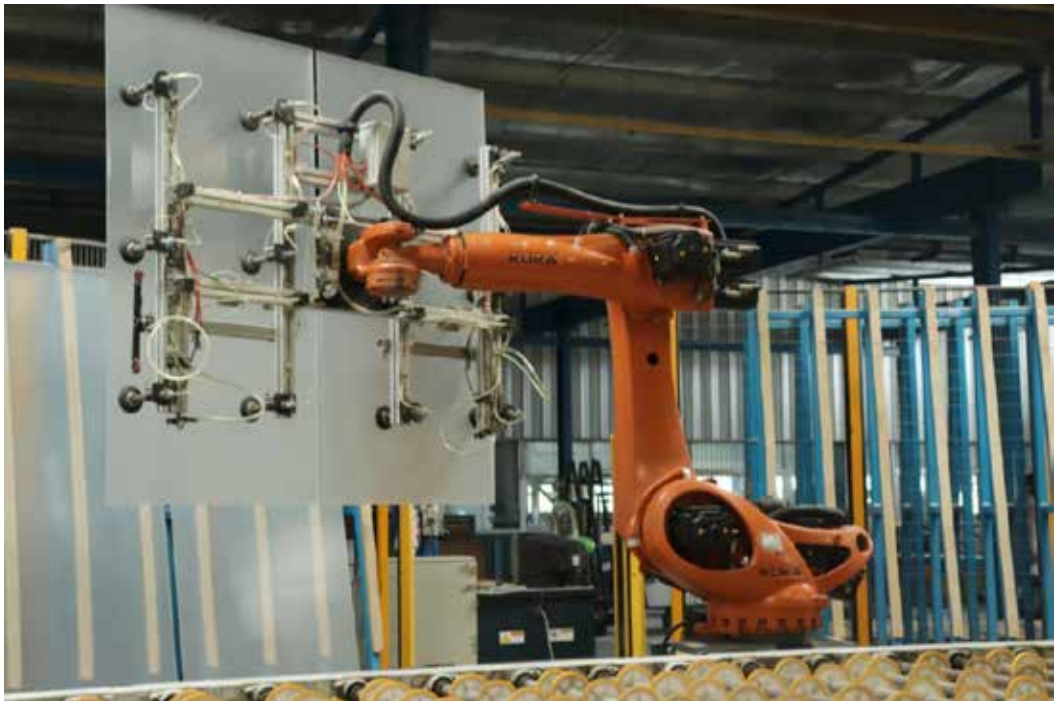
Automation in manufacturing process: Glass being lifted by a robot
