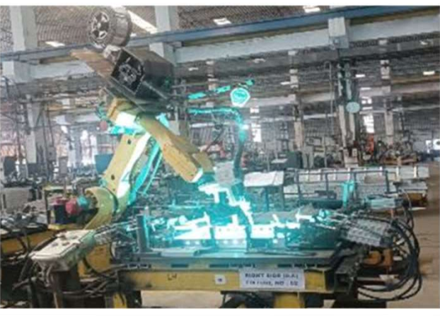
Robot at Mach one (Aluminium Welding)
