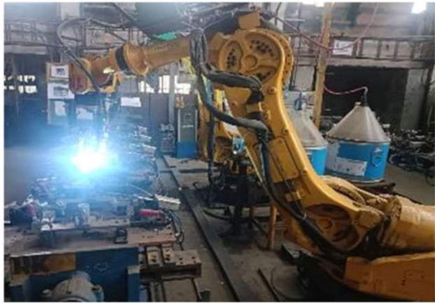
Robot welding at Scaffolding Dept.
