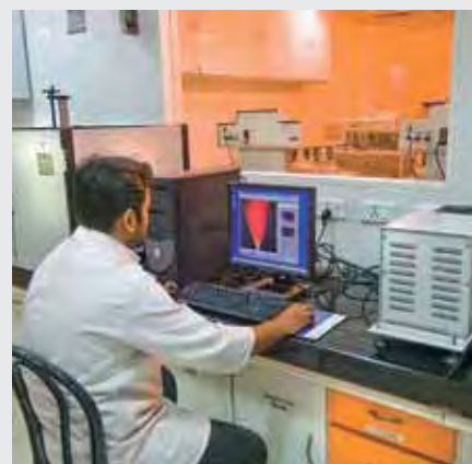
Plume geometry measurement of nasal spray
