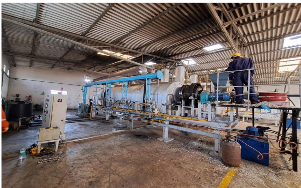
Workers Putting the Plastic waste in the machine to process it and convert it into Oil by the process of Pyrolysis
