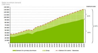
In 2019 total aluminium demand (Primary plus recycled) is projected to rise to around 90 million tonnes. While primary supply is likely to be around 65 million tonnes, about 25 million tonnes would be recovered from recycled scrap.
