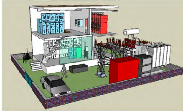
Compact 33 kV Distribution Station
