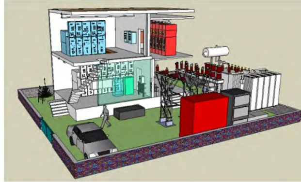
Compact 33 kV Distribution Station
