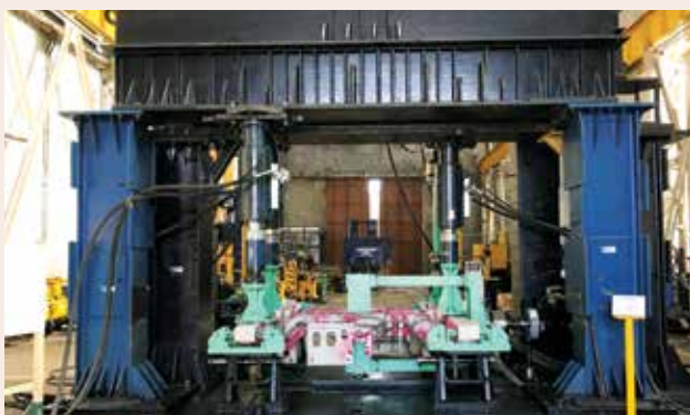
Static and fatigue test of RS13 Metro bogie frame as per UIC 615-4 requirements for DMRC at BEML R&D Facility by RITES.
