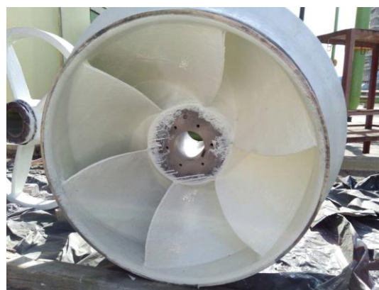
ANTI CORROSION COATING JOB
