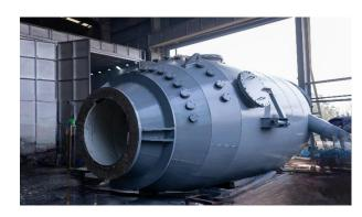
Material Hopper for Blast Furnace
