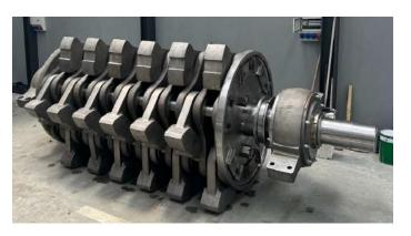
**Hammer Crusher Rotor**
