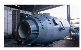
Material Hopper for Blast Furnace
