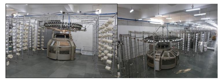
These Machines are employed in the knitting process to create the desired fabrics. Knitting machines are pieces of equipment used to knit textiles. A yarn bobbin feeds a variety of knitting techniques used in the production of the fabric. There are many diameter machines available, and each has a predetermined number of knitting sections. With a capacity utilization rate of roughly 92%, our 20 knitting machines can create 1500 tons of cloth annually.
