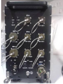
Datalink Systems \frac{3}{4} ATR •3U cPCI based •Supports Data Acquisition and Control
